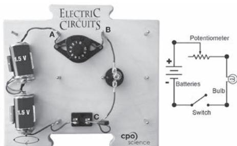
1. Build a circuit with two batteries, one bulb, the switch, and your potentiometer. Notice what happens when you turn the dial.
