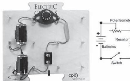
In this part of the investigation, your teacher will give you a **fixed resistor**. This component adds an unchanging resistance to the circuit. Replace the light bulb in the circuit from Part 1 with the fixed resistor as shown above.
