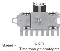
Remember, with one photogate, the timer measures the time that the beam is broken. As the car passes through the photogate, the light beam is broken for the width of the wing. The speed of the car is the width of the wing (**distance** traveled) divided by the time it takes to pass through the light beam (time taken). The advantage to this technique is that it is easy to move a single photogate up and down the ramp to make measurements of the instantaneous speed at many places.
