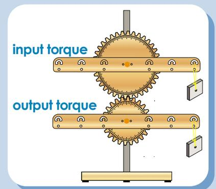
Stacking two gears or a gear and lever.
